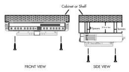
1) Choose an appropriate mounting location underneath a cabinet or shelf. Close proximity to an electrical outlet, TV antenna or cable connection will facilitate a neat, easy installation. Do not mount the VE720E/VE920E above a range or oven. Be sure that the location chosen will provide adequate access to the electrical connections on the rear of the unit before continuing.
